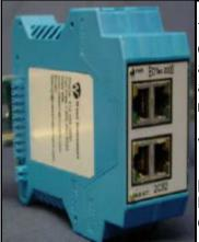
The 2C52 Ethernet 10/100 Base-T(X) Unmanaged Switch Module requires no user configuration. The data rate is automatically negotiated and the ports will auto-sense Full or Half duplex operation. The 2C52 will automatically learn the addresses of the devices connected to each port (up to 1024) and will buffer and route messages accordingly.
